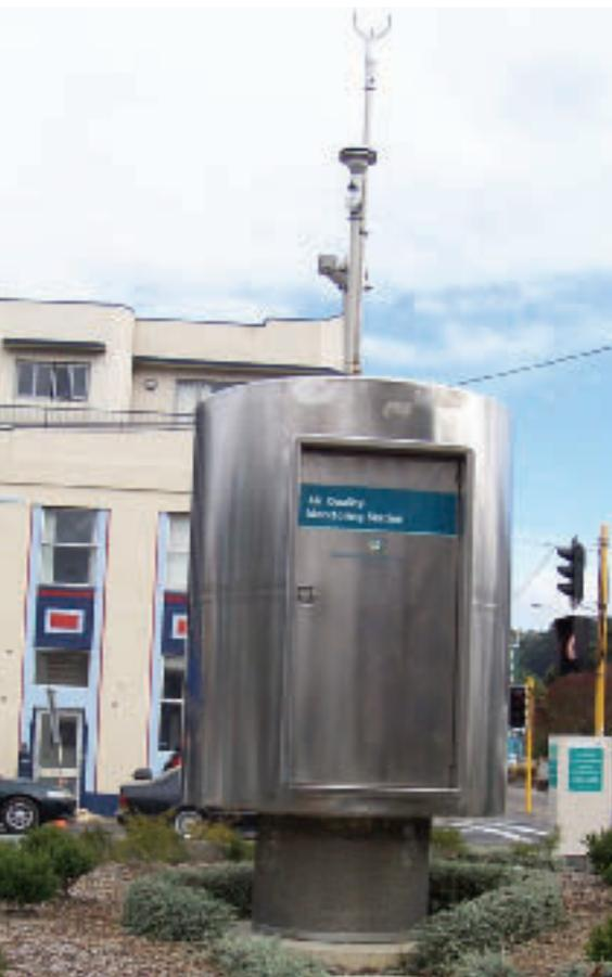
Permanent air quality monitoring stations like this one in inner city Wellington are continuously sampling the air for pollutants. This station also monitors air temperature, relative humidity, and wind speed and direction to help us interpret the results.
