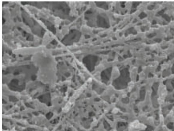
A filter we used to collect particles in winter at Masterton on 12 August 2004. Fine particle concentrations that day were measured at 77 micrograms/m<sup>3</sup>, exceeding the limit of 50 micrograms/m<sup>3</sup> set in the National Environmental Standard. The filter is completely coated – and your lungs would have trapped the same fine particles if you'd breathed in Masterton's air that winter morning.
