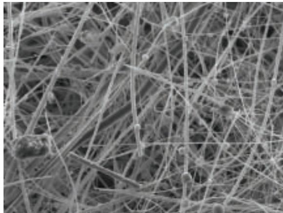
A filter we used to collect particles during summer – you can see a few particles here and there, mainly from wind blown soil, dust, seasalt and pollen.
