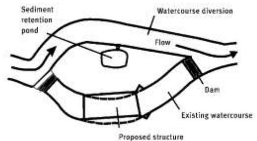
Figure 120: Dewatering construction area into a sediment pond
