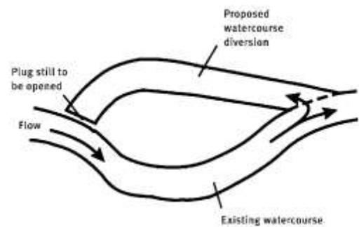
Figure 119: Diversion channel prior to plug removal
