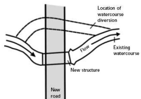
Figure 122: Re-establishment of flow in original channel
