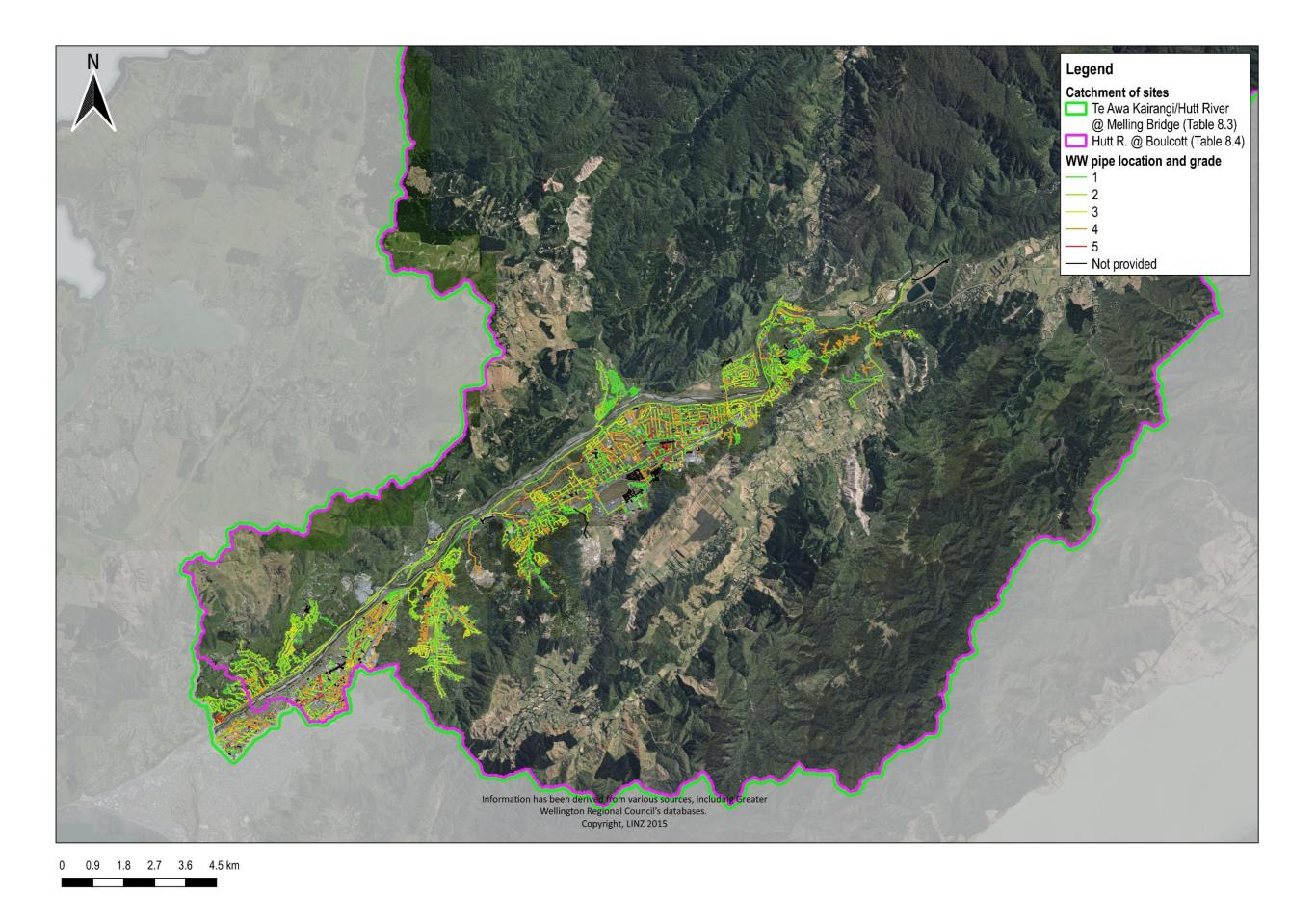
Figure 1: Location and condition of wastewater pipes upstream of the Te Awa Kairangi/Hutt River @ Melling Bridge primary contact site in Table 8.3 of PC1 and the Hutt R. @ Boulcott site in Table 8.4.
