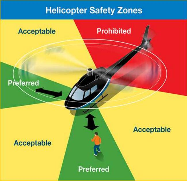
The diagram shows a helicopter with three safety zones: a red 'Prohibited' zone behind the tail rotor, a green 'Preferred' zone in front of the rotor hub, and yellow 'Acceptable' zones to the sides and in front of the tail. Arrows indicate the direction of rotor rotation.
