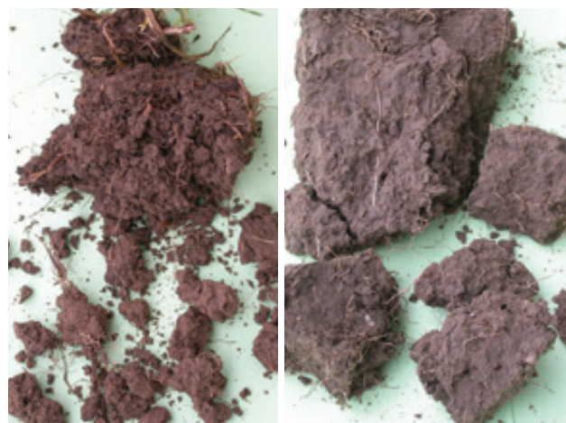
Figure 2: Non-compacted soil (left) and severely compacted soil (right)
