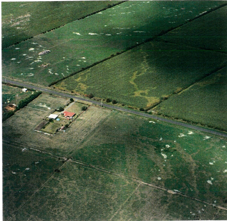
Photo 3. Aerial view of sand boils near Powell Rd.
