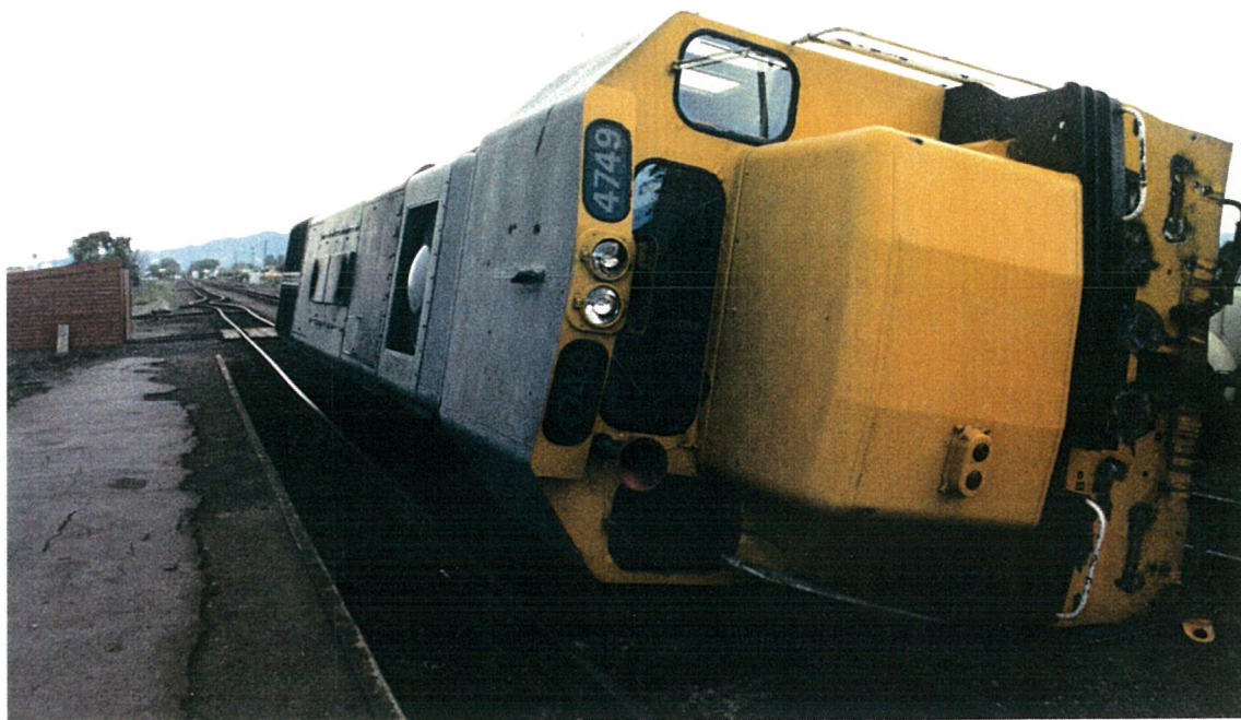
Photo 10. 67 ton diesel locomotive toppled in Edgumbe.
