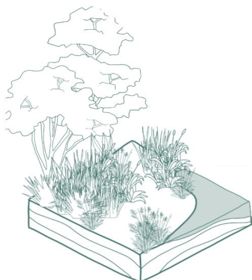
Figure 8.3: Whānau planting for channel realignment and floodplain re-engagement – clustered awa corridor planting, both wet and dry typologies, low maintenance and robust planting.
