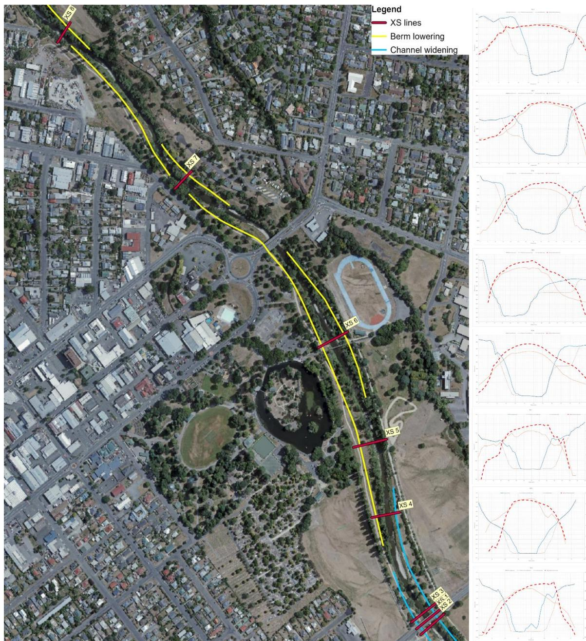
Figure 1.1: Extent of berm lowering in lower Waipoua through Masterton (yellow lines on aerial photo) in conjunction with cross-sections (red lines on aerial photo). Modelled velocities in orange (existing cross-sections) and red dashed (modified cross-sections) lines shown alongside image. In all sections except XS 8 lowering of the berm increases velocities. All velocities exceed critical velocities for entrainment and transport of gravel (cf. Figure 1.3)
