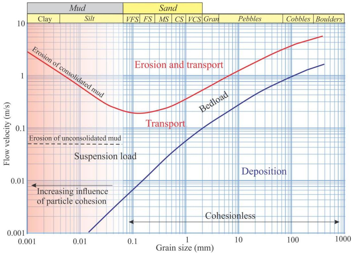
Figure 1.3: Hjulström Curve, plotting the relationship between flow velocity and entrainment/transport/deposition of grain sizes ranging from clay to boulder. The critical velocity for entrainment of particles of a given size is delineated by the red line. Entrainment velocities are higher than transport velocities. Note: the critical velocity for entrainment of gravel is around 1 m/s
