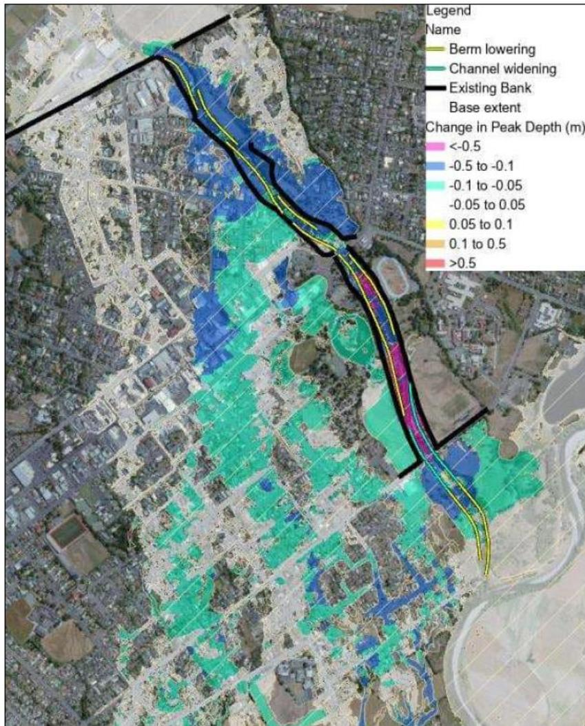
Figure 1.2: Depth difference layer for a 1% AEP flow ( $Q_{100}$ ) between the base scenario and LRS combined option 13 (channel widened and berms lowered), source: Land River Sea Consulting Limited Memorandum to Greater Wellington Regional Council, 13 September 2024, Figure 2-22
