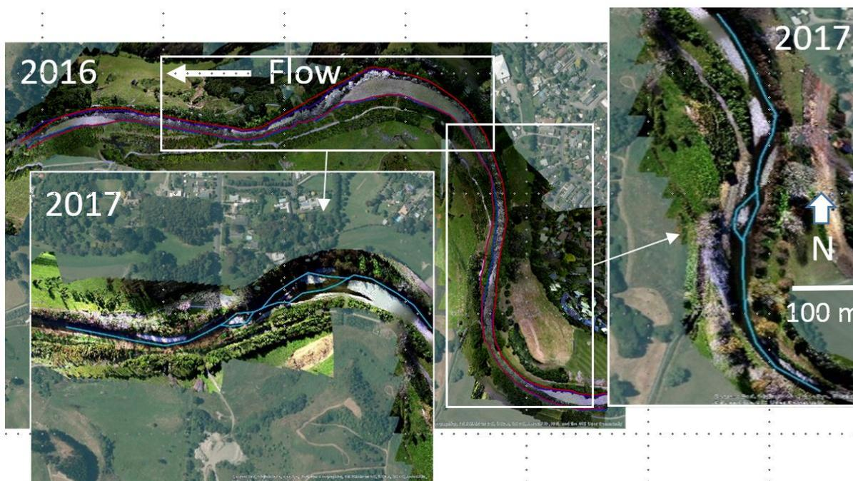
Figure 1.6: Changes in the Waikanae River at Jim Cooke Memorial Park following widening in 2017 (from Fuller et al., 2021<sup>2</sup>)
