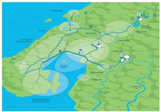
This diagram illustrates the bulk water supply pipes that Greater Wellington owns and maintains.
