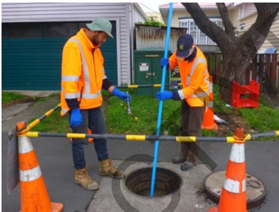
Using the extendable-handle kick net to collect a macroinvertebrate sample
