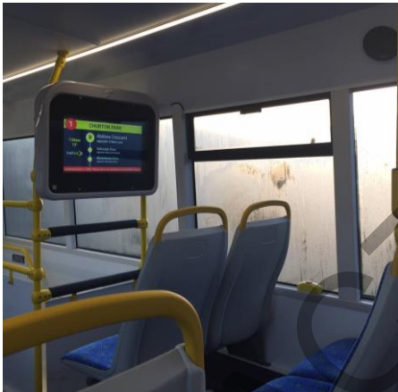
Fig 1: Condensation on windows in daytime
