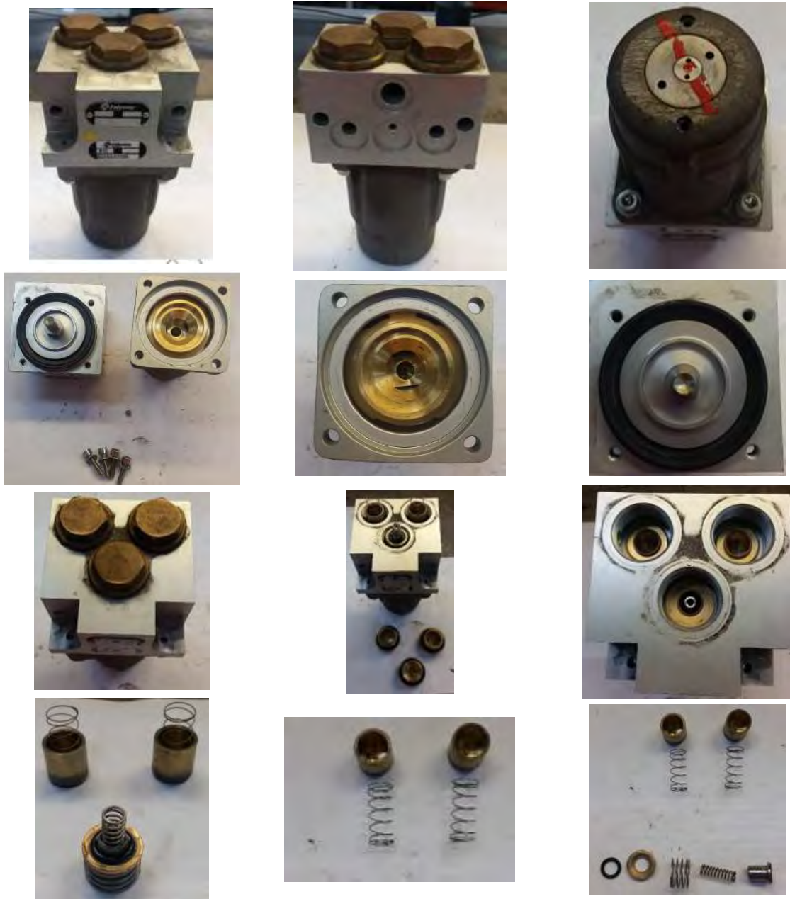
Figure 4 – Depicting Strip Down of NJMR – Spring Reference Distributor SN. 005
