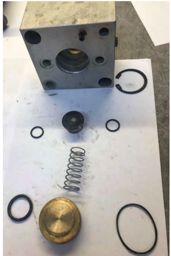
Figure 16 – Depicting Strip Down of Pressure Reducing Valve – SN: 641
