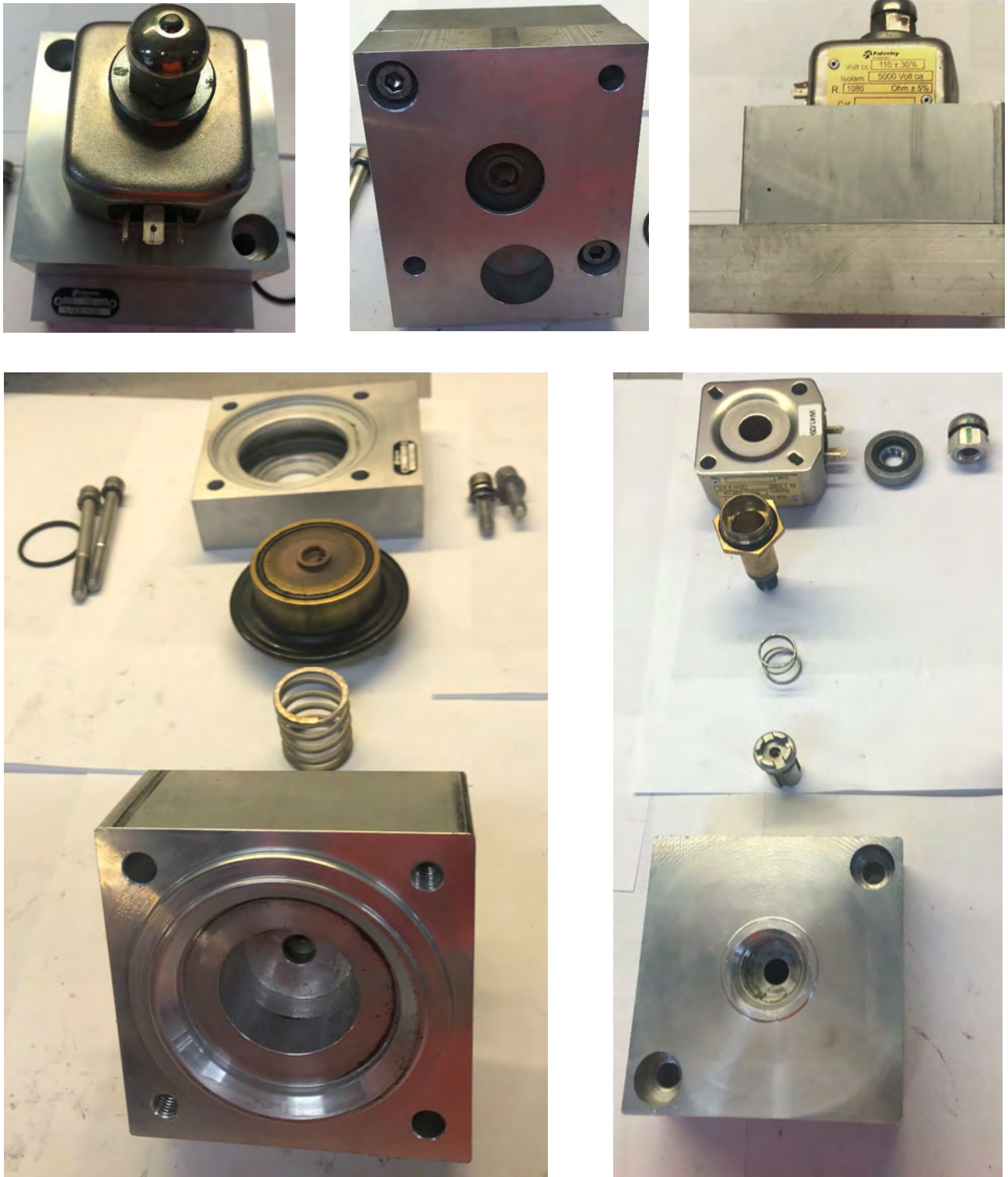
Figure 15 – Depicting Strip Down of Emergency Application Valve – SN: 82
