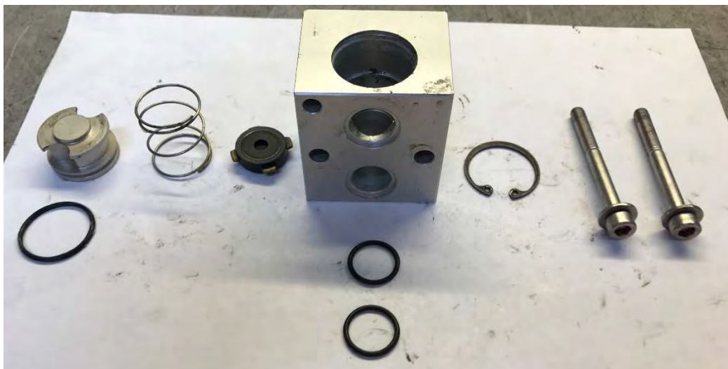
Figure 9 – Depicting Strip Down of Check Valve – NP: 4206
