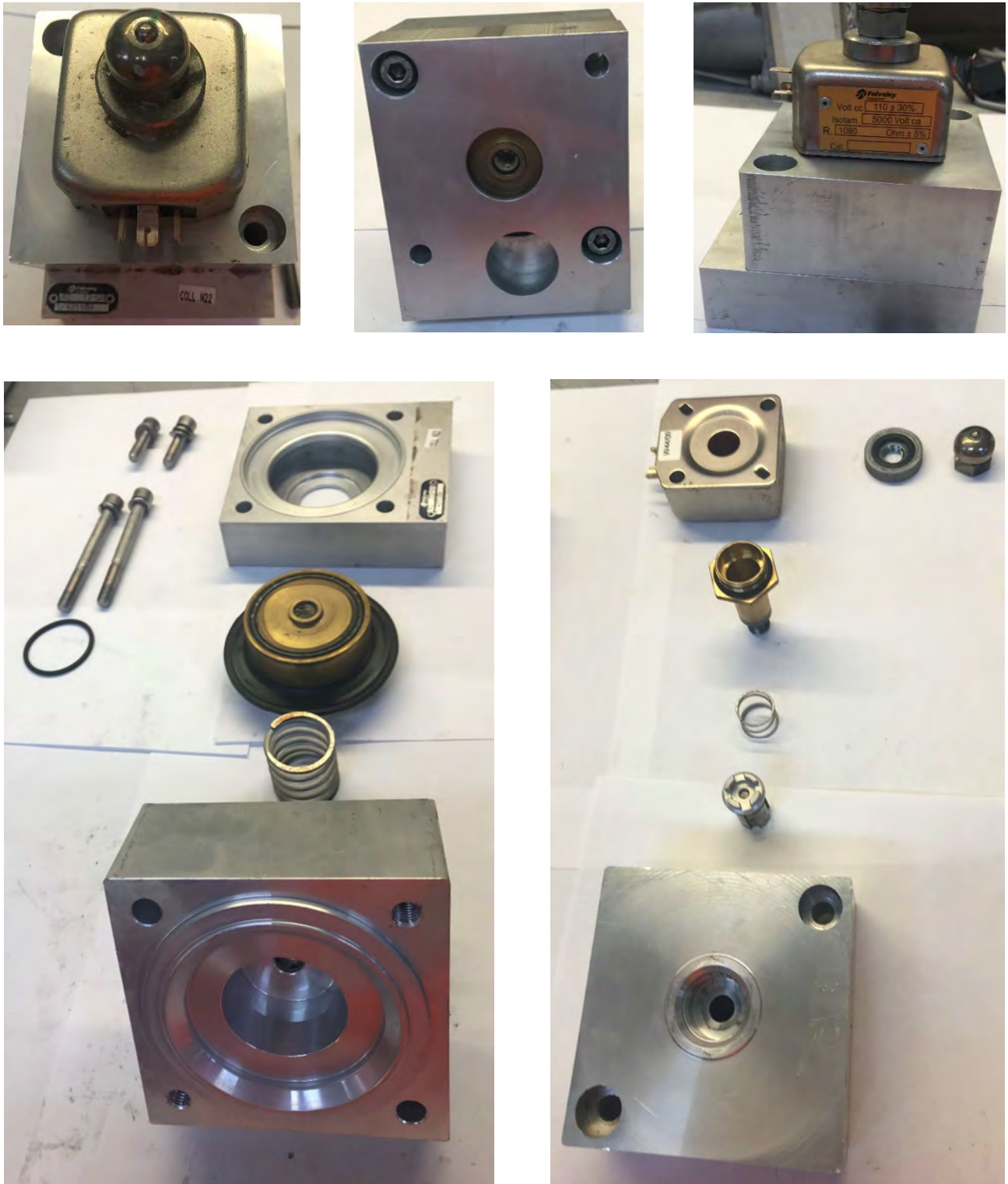
Figure 14 – Depicting Strip Down of Emergency Application Valve – SN: 92
