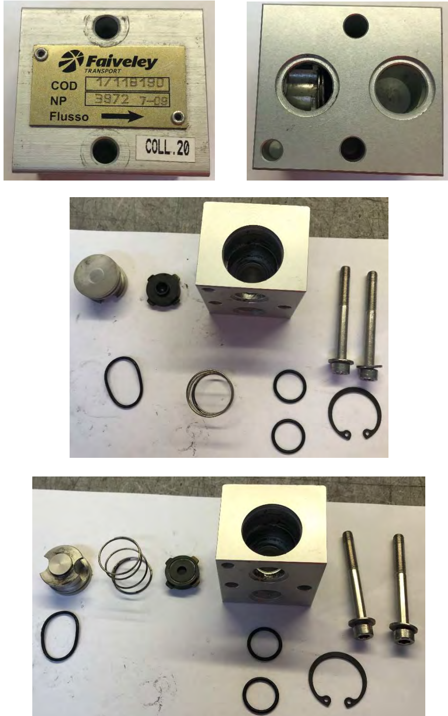
Figure 4 – Depicting Strip Down of Check Valve – NP: 3972
