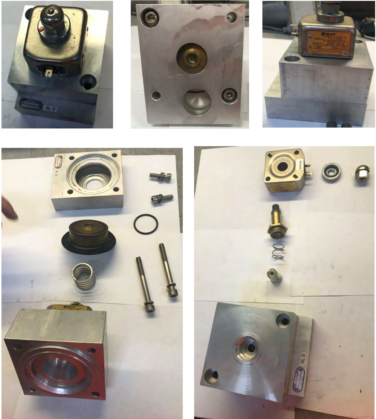
Figure 12 – Depicting Strip Down of Emergency Application Valve – SN: 57
