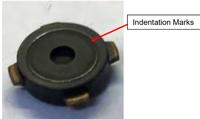
Figure 19 – Depicting Indentation Markings of ‘Valve Complete’
