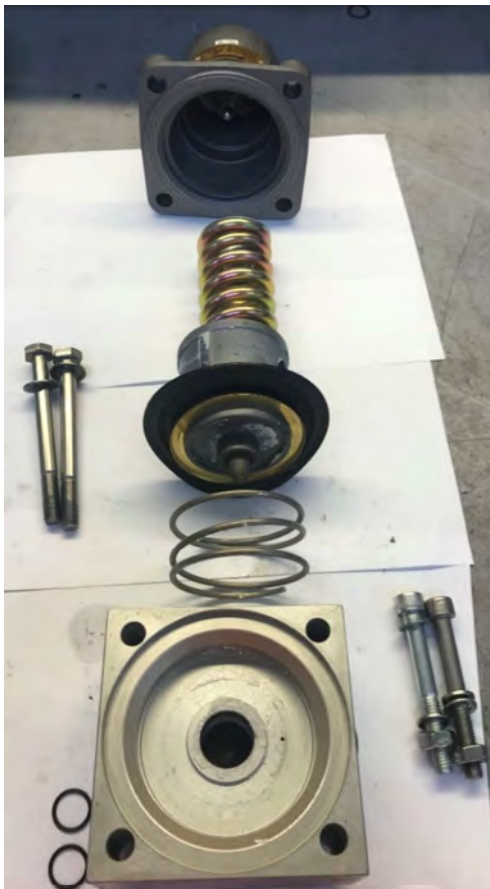
Figure 16 – Depicting Strip Down of Pressure Reducing Valve – SN: 641
