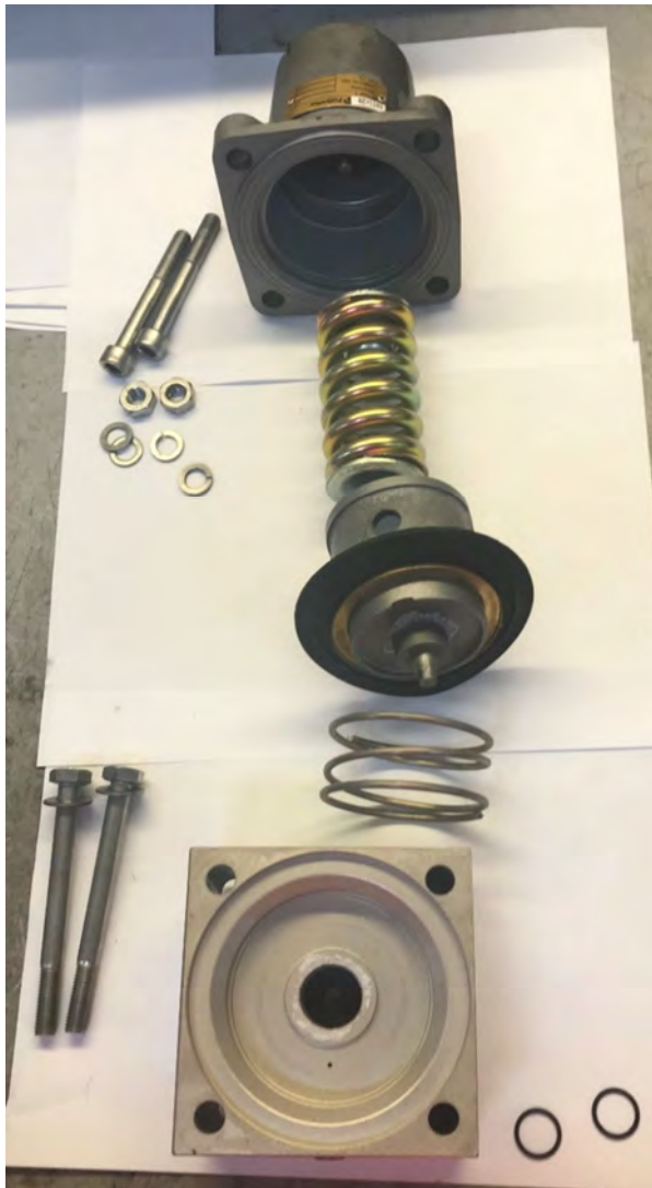
Figure 17 – Depicting Strip Down of Pressure Reducing Valve – SN: 654
