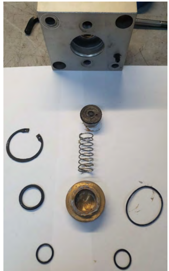
Figure 18 – Depicting Strip Down of Pressure Reducing Valve – SN: 656
