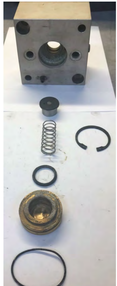
Figure 17 – Depicting Strip Down of Pressure Reducing Valve – SN: 654
