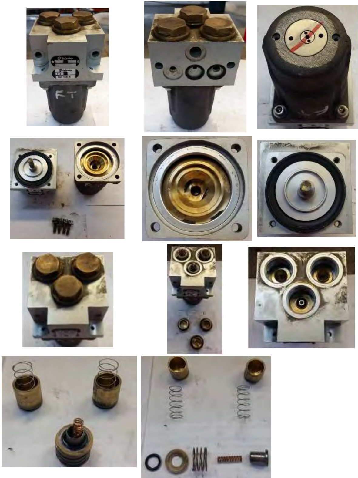
Figure 5 – Depicting Strip Down of NJMR – Spring Reference Distributor SN. 035
