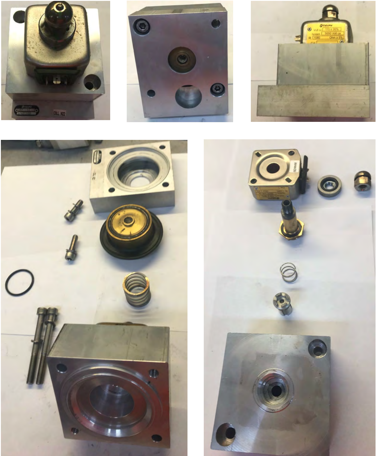
Figure 13 – Depicting Strip Down of Emergency Application Valve – SN: 87
