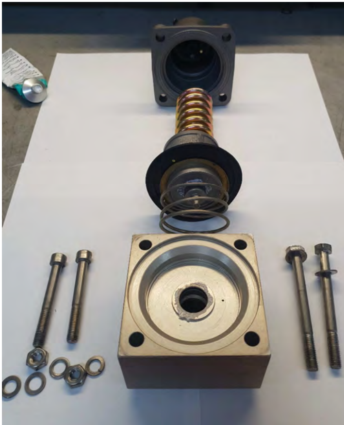
Figure 18 – Depicting Strip Down of Pressure Reducing Valve – SN: 656
