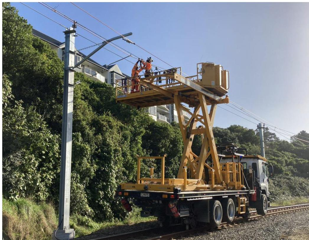
*Easter Block of Line Activity- Raroa Station pedestrian bridge and ongoing removal of redundant traction masts and defect remediation*
