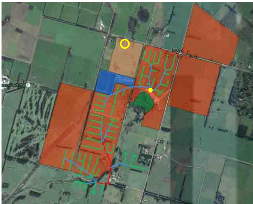
Figure 9: Existing Irrigation Layout, Existing bore (yellow dot) to be decommissioned and Existing dwelling (yellow circle) to be relocated.
