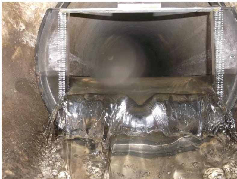
Figure 20: Night flows observed in the early hours of the morning during night flow isolation I&I investigations (note clarity of sewer flow)
