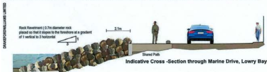
Simulated view of proposed shared path with rock revetment protection works in Lowry Bay
