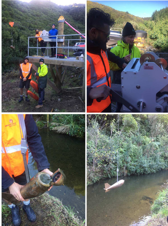
L-R (top) Aquatic team check the new platform, Wendy shows Shyam how to use the winch. L-R (bottom) up close of sediment bomb and sediment bomb being deployed.
