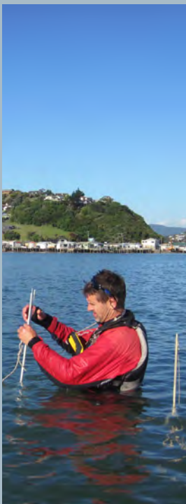
Measuring frame and probe used to measure shallow subtidal plates.
