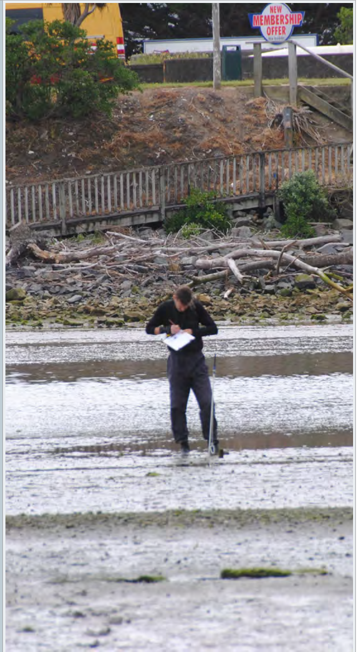
Measuring sediment plates in the lower Hutt Estuary, Jan 2017.
