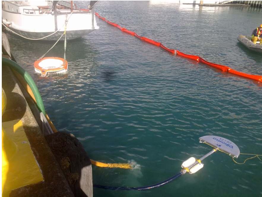
A floating harbour containment boom and floating skimmers.
