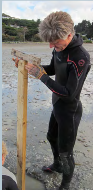
Installing and levelling a sediment plate in Browns Bay, January 2013.
