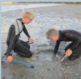
Installing and levelling a sediment plate in Browns Bay, January 2013.
