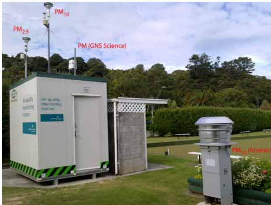
Figure 1.1: Photo of GWRC monitoring station showing sample inlets for particulate matter monitoring instruments and the high volume sampler (right foreground)
