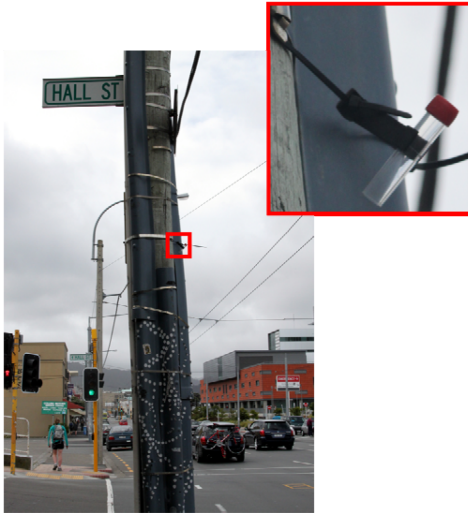
Figure 4.3: Location of passive nitrogen dioxide monitoring tubes (red square) at NZTA's monitoring site on the corner of Riddiford and Hall streets, Newtown, Wellington
