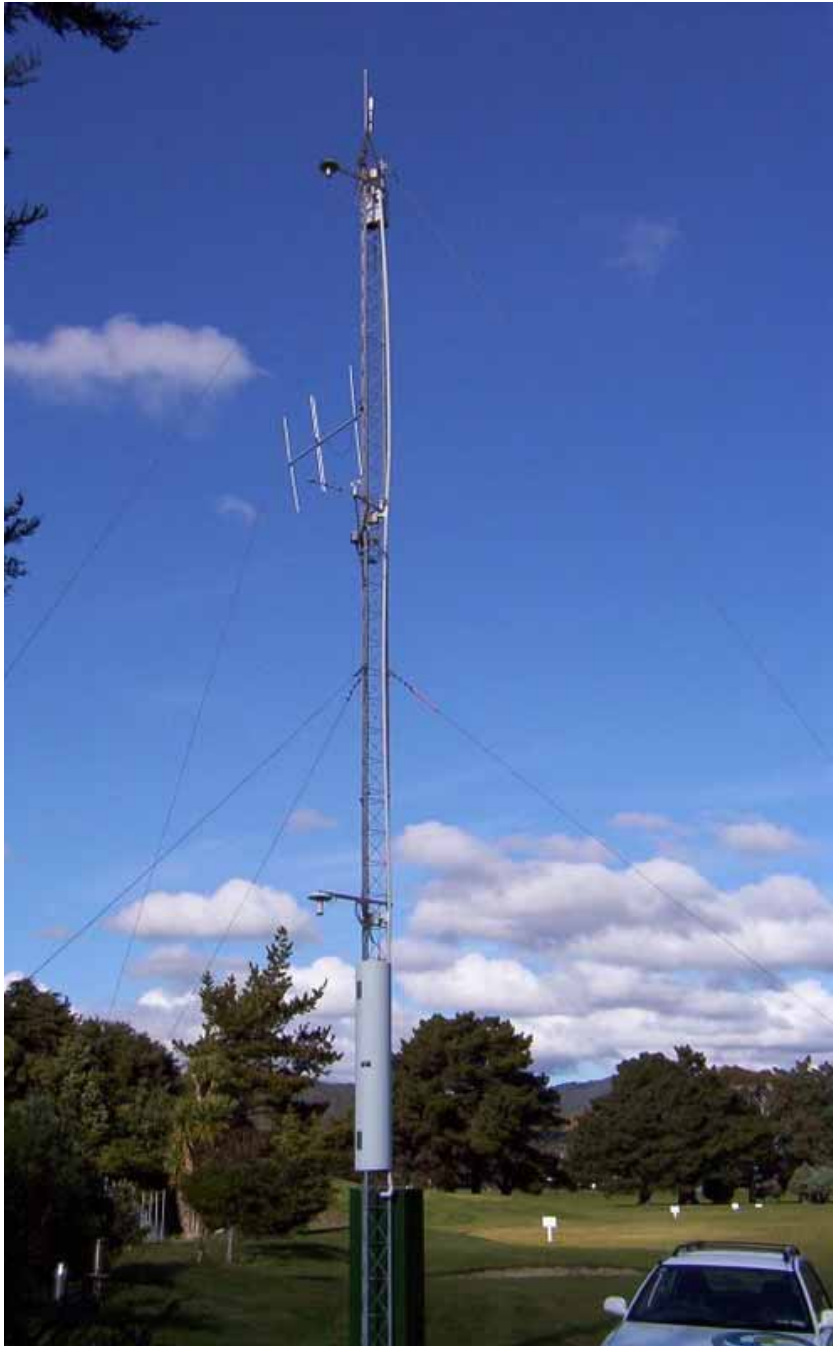
Figure 2.3: Greater Wellington meteorological monitoring station with 15 m mast located at Shandon Golf course, Petone
