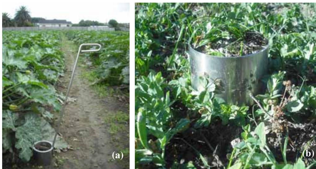
Figure 2.2: (a) Collecting a composite of core samples along a transect using a soil corer. (b) One of three intact core samples taken at each site, to establish the physical properties of the soil.
