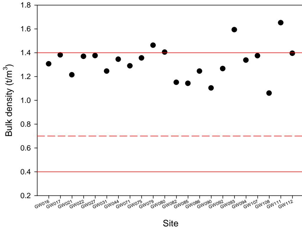
Figure 3.2: Bulk density at each soil quality monitoring site sampled over 2009/10. The area between the red lines represents the optimal range\*.
