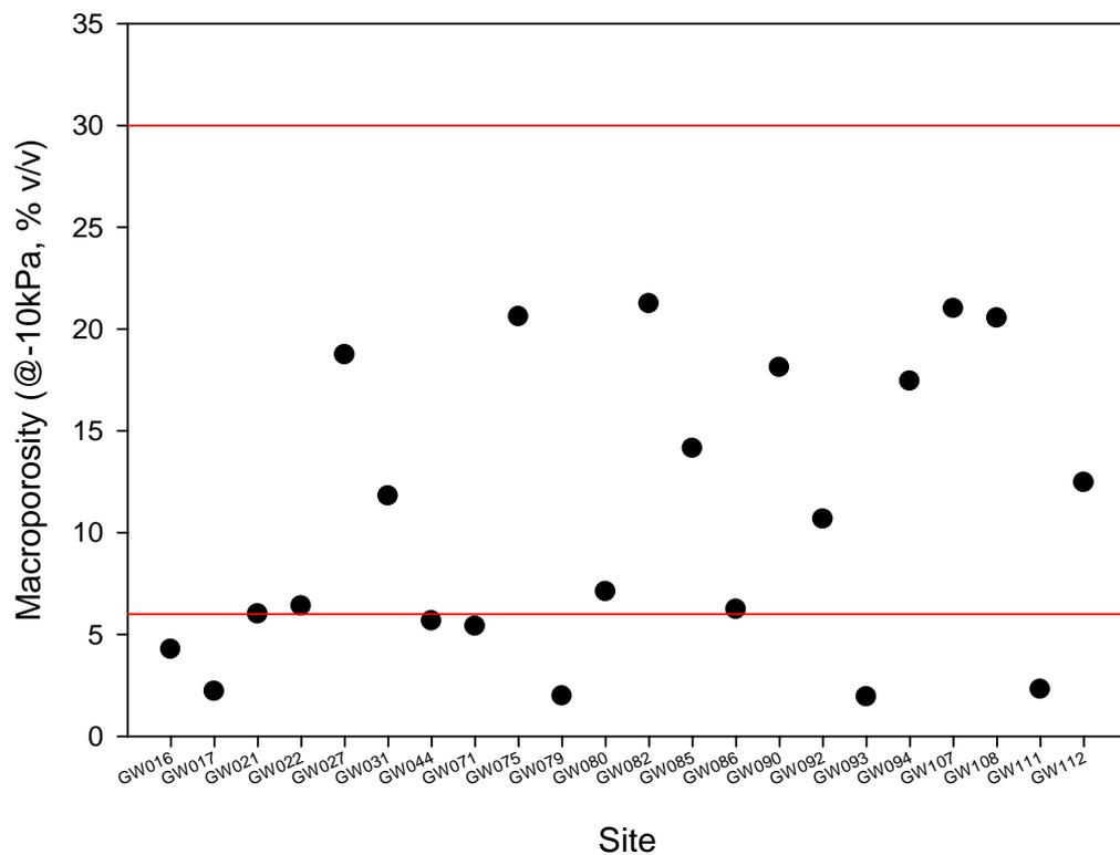
Figure 3.3: Macroporosity at each soil quality monitoring site sampled over 2009/10. The area between the red lines represents the optimal range.
