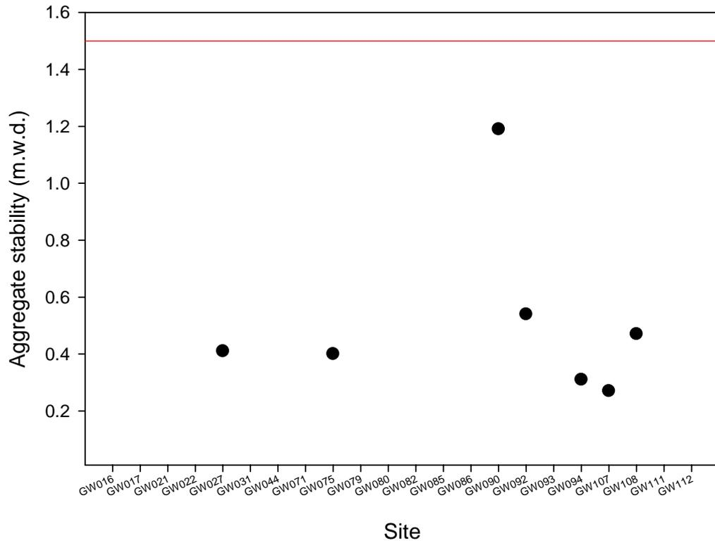
Figure 3.4: Aggregate stability at seven market garden soil quality monitoring sites sampled over 2009/10. The red line represents the lower limit for good soil structure, and the level at which production will begin to decrease.
