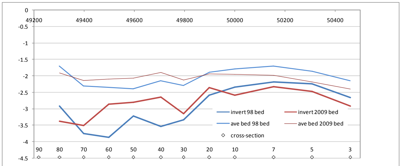
Figure 2 Bed levels for 1998 and 2009 surveys
