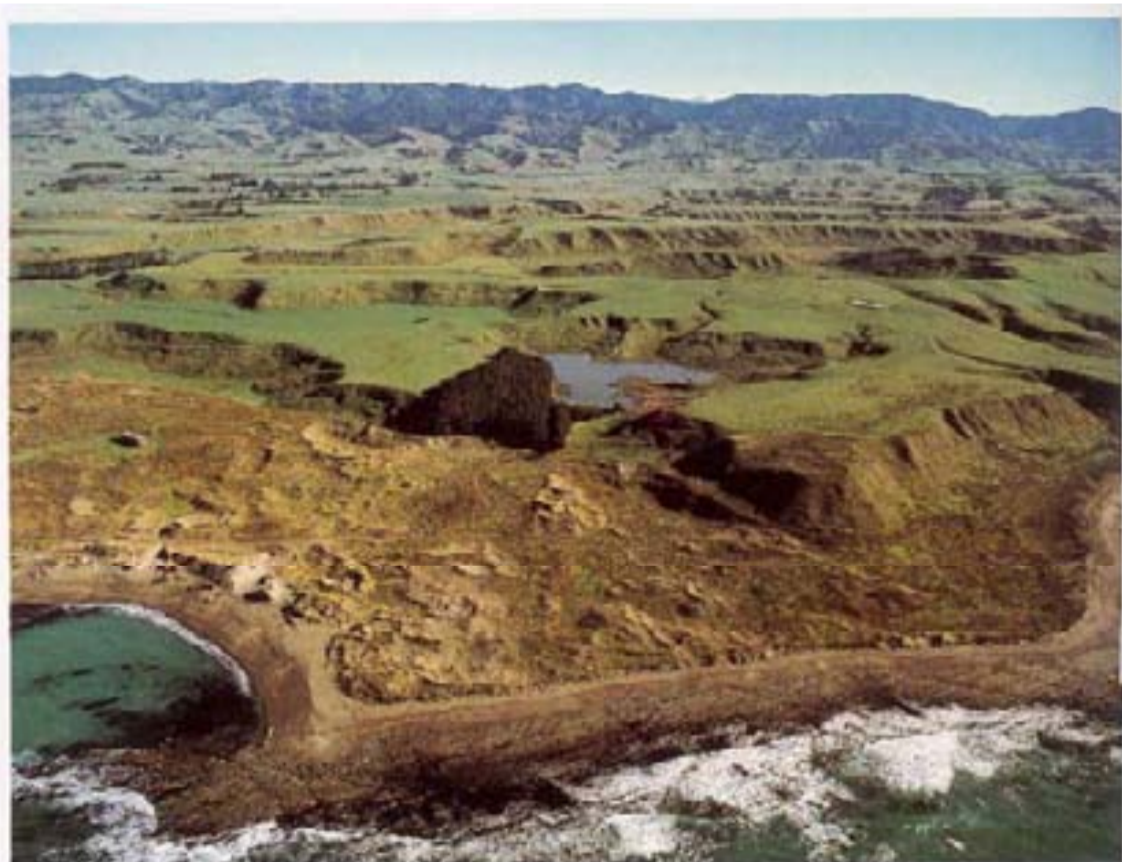
Figure 29 Elevated, dissected terraces are extensive between Uruti Point and Flat Point and the hills of the eastern uplands. The terraces are underlain by marginal marine sand and gravel and are interpreted as the last interglacial (O1 5) marine bench. The bench is 15–20 m above today's mean sea level here at Uruti Point (T27/672039), but rises to more than 80 m at the Kaiwhata River mouth, indicating that active uplift is occurring along the coast, and that uplift is faster in some areas than others. The marine bench, near horizontal when cut, now dips gently to the west in the Uruti Point area, showing that the Whararama syndine is actively deforming. The surface is also disrupted by the Flat Point Fault, particularly in the Kaiwhata River area. The seaward edge of the O1 5 marine bench is marked by a cliff eroded by the sea in the mid Holocene. Extensive Holocene sand dunes overlie alternating beds of the Whakataki Formation.
