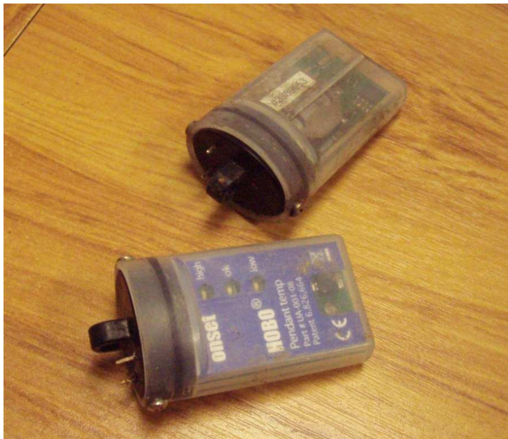
Figure 2: Loggers placed in the stream beds at intermittent sites to record the presence/absence of water at daily intervals.
