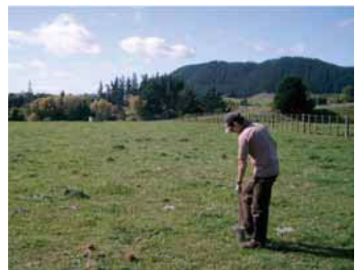
This dairy farm in Otaki is one of our soil quality monitoring sites. At each monitoring site, samples are taken from a depth of 0-10cm using a soil corer (pictured above), tested for various indicators, and the results compared with the optimum range for the soil type and land use. The soil at this site was slightly compacted but nutrient levels were satisfactory.
