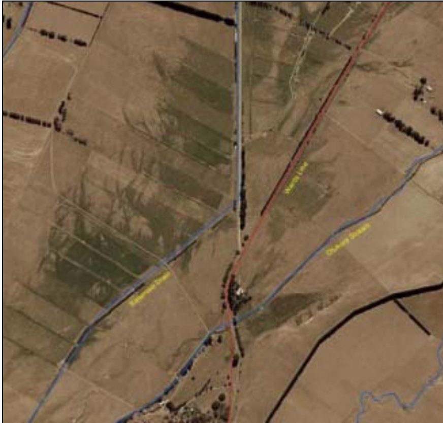
Figure 12: Aerial photograph showing the effect of subsurface irrigation from the Battersea Drain, during summer 2001/02.
