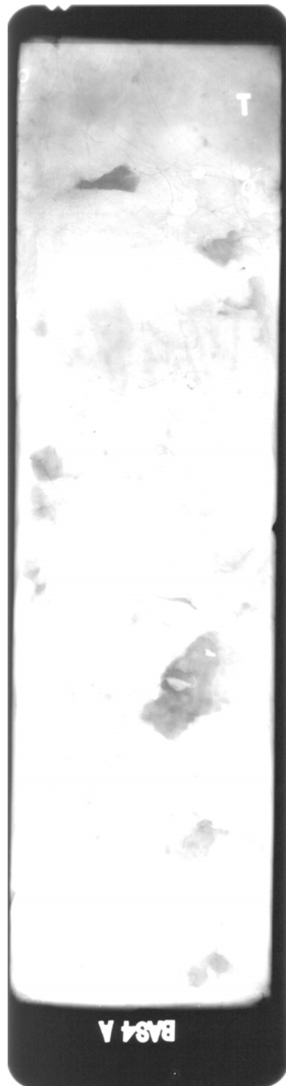
Figure A16: Basin Site Four (BAS4) short-core x-radiograph of 2-cm thick slab. Exposure: 50 kV, 25 mA, 2 minutes. Scale: core width is 10 cm, length is 40 cm.
