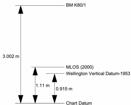
**Figure 4:** Relationship between datum levels at the Queens Wharf site. MLOS (2000) is the mean level of the sea reported by LINZ in 2000. Another longer-period estimate of MLOS by LINZ is 1.08 m averaged over the 18-year period 1989-2007.<sup>4</sup>
