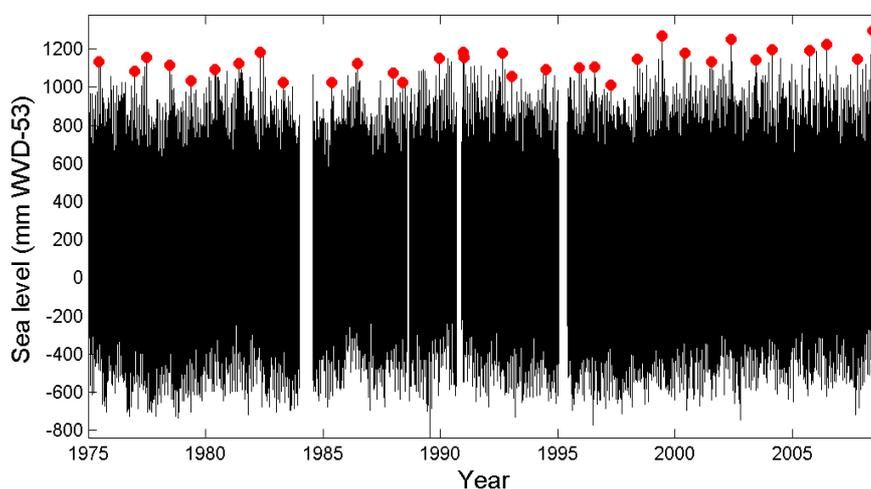
**Figure 5:** Wellington sea level measured at Port of Wellington, relative to WVD53. The Annual Maxima (largest sea levels for each calendar year) are marked by the red dots.
