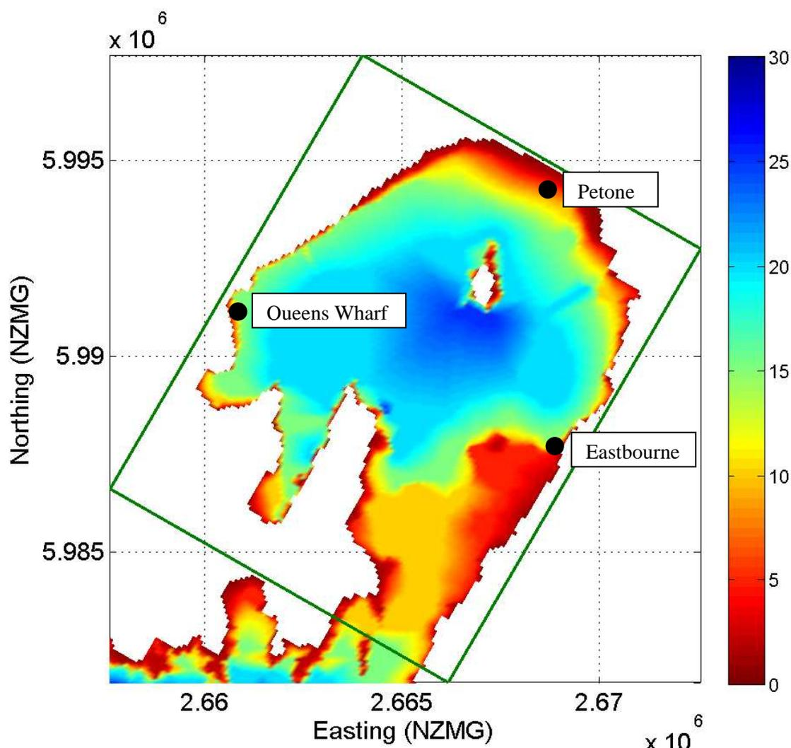
**Figure 8:** Bathymetry of Wellington Harbour illustrating the model grid area, which was subsequently orientated  $30^\circ$  relative to True North. Model output sites at Queens Wharf, Petone and Eastbourne are marked.
