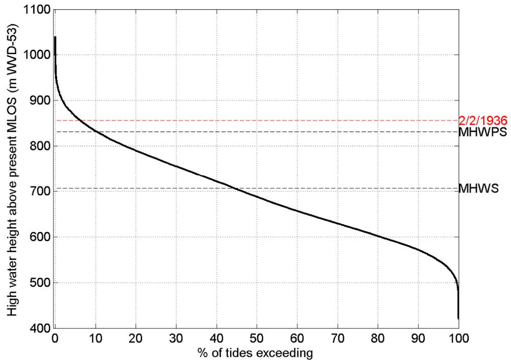
**Figure 1:** High tide exceedance curve based on the tidal component of the Wellington sea level record (see Figure 6). Also shown are MHWS = Mean high water springs Scientific (when  $M_2 + S_2$  combine over a fortnight) and MHWPS = mean high water perigean springs (when  $M_2 + S_2 + N_2$  combine over 6–7 months) levels, along with the back-predicted high tide level at 00:15 on 2 Feb 1936. MLOS = mean level of the sea.
