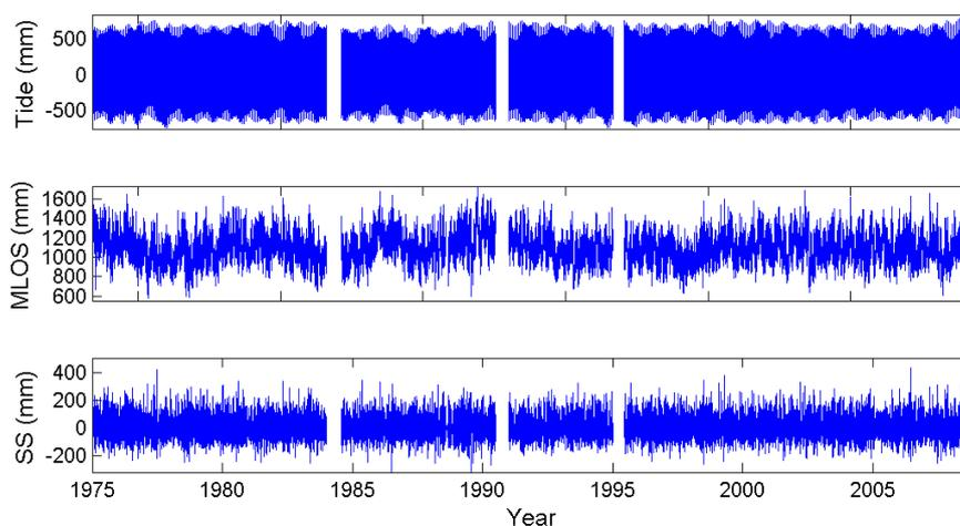
**Figure 6:** Components of the Wellington sea level record (mm relative to WVD53). MLOS = Mean level of the sea, SS = storm surge.
