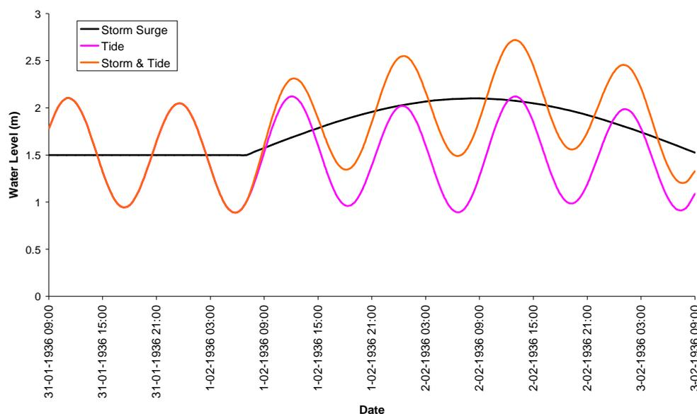
**Figure 9:** Boundary conditions used to force the MIKE 21 storm surge model. The vertical datum for the plot is Chart Datum.
